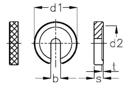
$\begin{array}{lll} b & = 10.4 \\ d1 & = 34 \\ d2 & = 25 \\ For bolt = M10 \\ s & = 8 \\ t & = 1.2 \end{array}$
